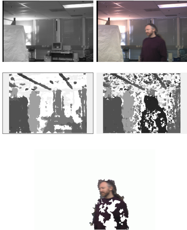
Figure 2. Middle images show range background model and new scene image. Stereo computation can not produce valid range estimates in areas which have very low texture (e.g. saturated regions) or which are occluded in one view. Invalid range values are shown in white. Depth based segmentation, shown in bottom image, will fail in regions of the foreground which are undefined in depth. Top row shows color background model and scene image for reference, although they are not use in segmentation. Color of the foreground is overlaid on the segmentation results for easier interpretation.
